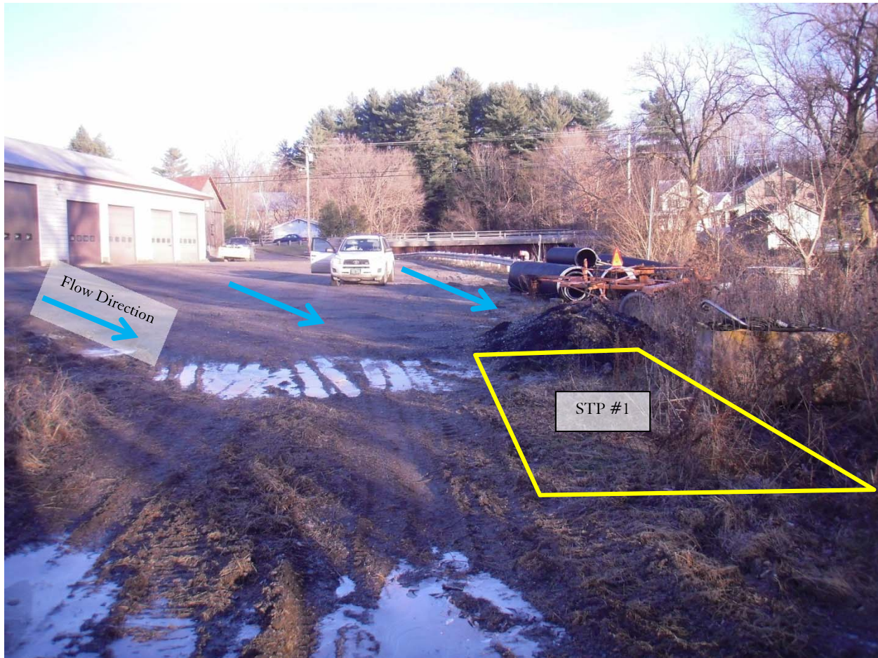
Figure 3. Stormwater that currently flows, southwest across the property could be captured and treated in an STP in the southwest corner of the property.
