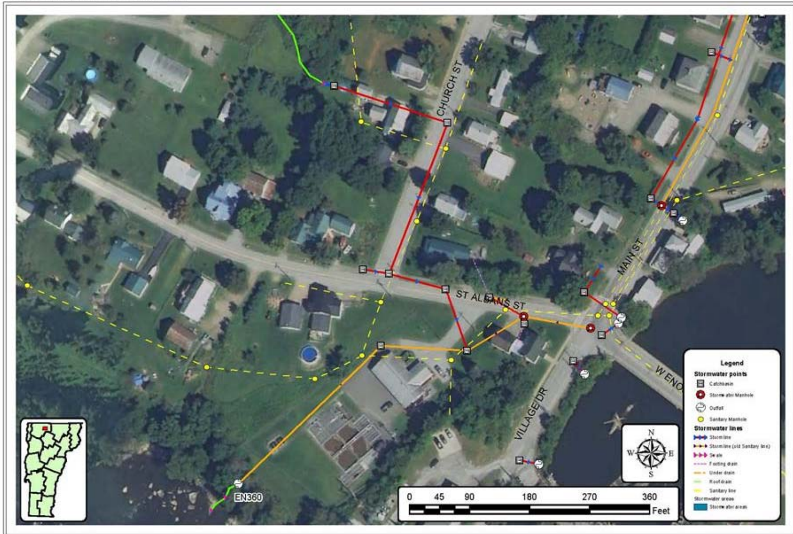
Figure 3. Stormwater drainage system discharging at outfall EN-360 Enosburgh Falls, VT
