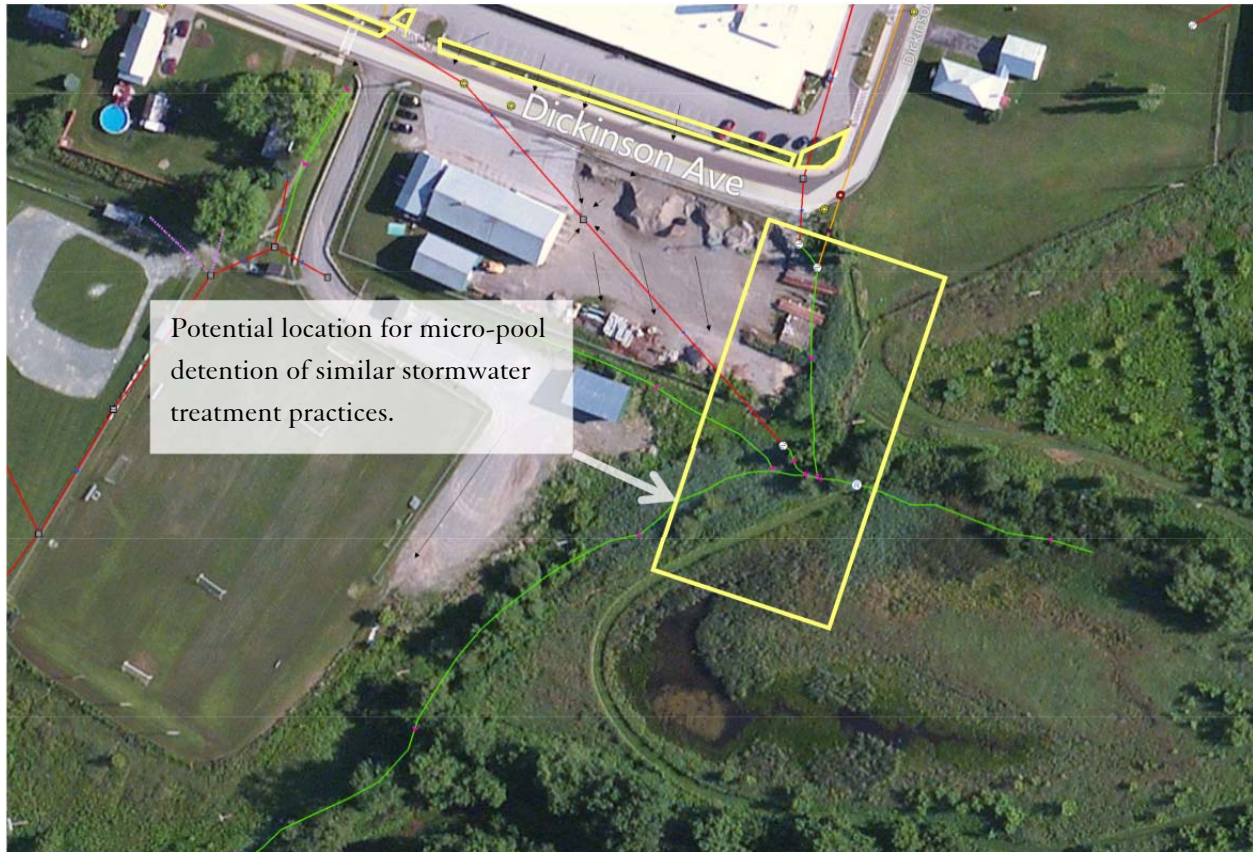
Figure 16. Possible location of proposed STP southeast of the Enosburg Falls road maintenance yard.
